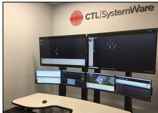
The Central Monitoring System displays the Spectrum Patrol Software, and features the ability to operate in a multi-display setup showing simultaneous results of Spectrum Patrol's multiple capabilities.
